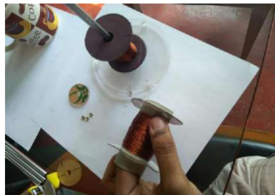
Figure 2: Coil winding on a handmade cardboard
