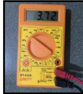
Figure17: Battery voltage after the battery charge by shock absorber model
