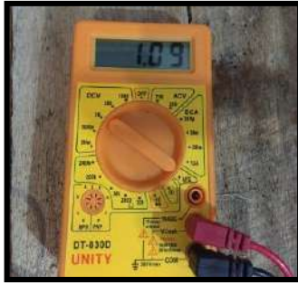
Figure 16: Battery voltage Before the battery charge by shock absorber model
