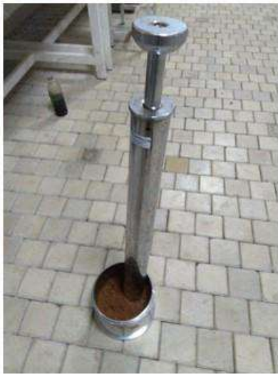
Image 09 & 10- Sample preparation of CBR Test
