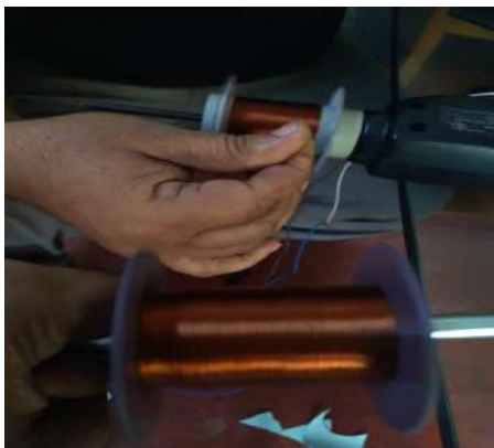
Figure 1: Coil Winding using drilling machine
