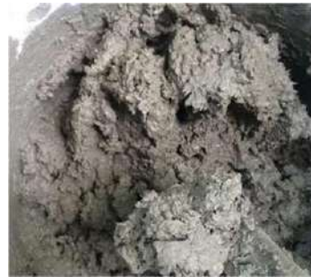
Figure 3: Paper Cement Mixture
