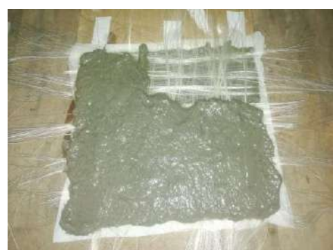
Figure 7: Adding second layer after layering fibers
