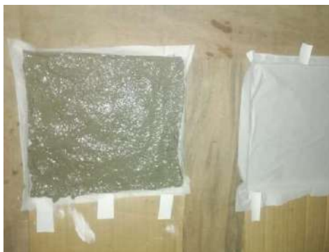
Figure 6: Adding first layer of 2.5mm
