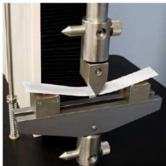
Figure 10: 3-point flexural test arrangement
