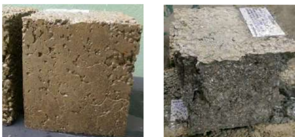
Figure 2: G1 - 0.4 W/C test specimen
