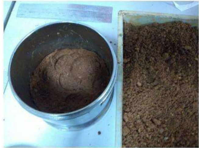
Image 09 & 10- Sample preparation of CBR Test
