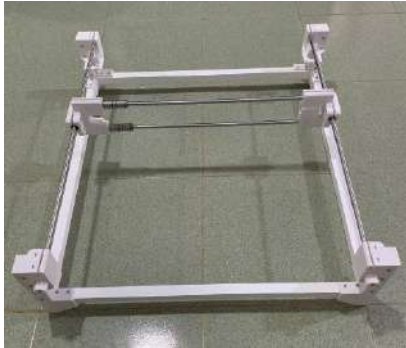
Figure 5 - Basic Frame Structure
