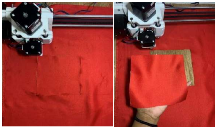
Figure 9 - Before and after the pattern was cut out using the machine
