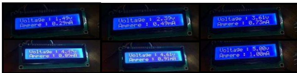
Figure15: Different voltages and amperages displayed when pressing the shock absorber model in different speeds
